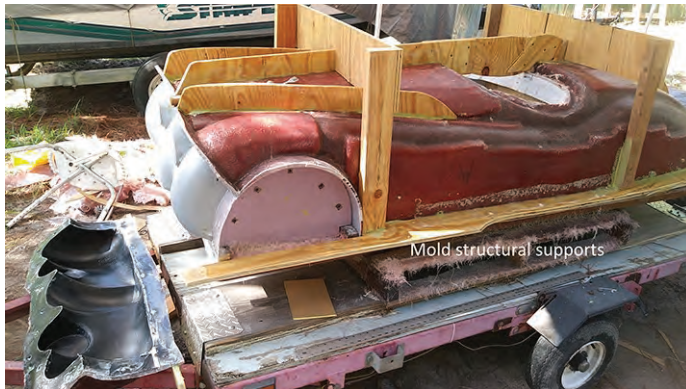
Mold complete with reinforcements before trimming
