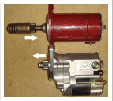
The new high torque starter operates very differently. When this starter is energized, first a solenoid is energized. This moves the gear in the direction shown above to engage with the flywheel gear. When they are engaged, electrical connection is made to the starter motor and the gear turns, spinning the engine. This is like most modern cars.
