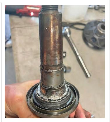
The outer bearing had been destroyed, the bearing spacer had galled to the axle, the inner bearing was junk, etc., so online parts diagrams were referred to, cross-checking of parts and quantities confirmed, and the old axle was put back in. Sure, the wheel was loose and wobbled because the bearing was missing, but still, it was progress! Now the car can be rolled out of the garage while parts are ordered. Next month we should have the repair complete.
