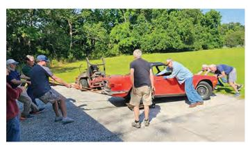
So, we placed the floor jack under the differential and while pulling the jack and people pulling and pushing the car, we were able to get it in place to be raised by the lift.
