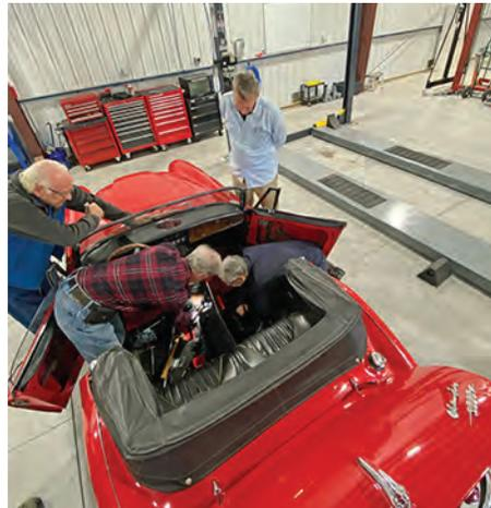
Anyway, with the transmission exposed we unbolted the driveshaft and, fortunately, it easily moved back out of the way. Dave had brought a 32mm socket that fit the nut to remove that and gain access to the coupling flange. All that came out nicely and with a new tool Dave had purchased from **Harbor Freight** the old seal was out. Checked the fit of the new \$2.59 seal, oiled it up and
