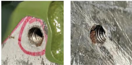
So, a couple of **Heli-Coils** were installed:
