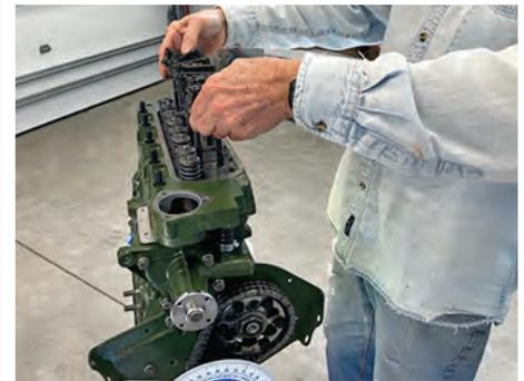
We realized that the new crankshaft pulley / dampener does not have a timing mark, which strikes me as odd. A quick search shows that **Speedwell Engineering** makes a kit based on the **1968 Works BMC Le Mans** timing pointer that moves the pointer & marks up to where you can actually see them, so we are on hold waiting for that to arrive. 🇬🇧
