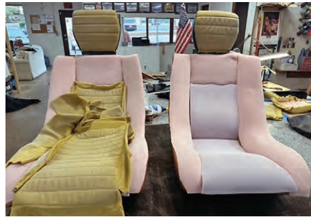
Checking width of new bolsters against the fabric insert.
