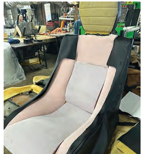
Checking width of new bolsters against the fabric insert.
