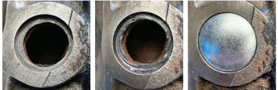
Installing new freeze plugs following the usual process; clean the seat for the plug, apply black RTV, and hammer in the plug.
