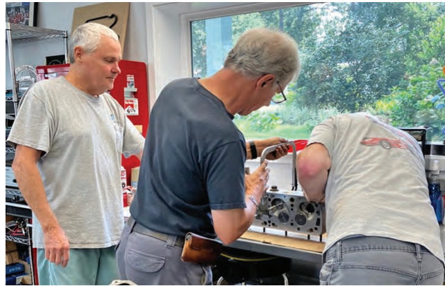
Dave operates the valve spring compressor while Gene and Frank drop in the collets.
