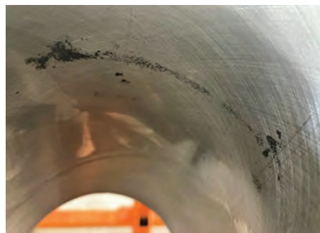
Well, here's a reason to have a lot of light in the shop – the corrosion in the #3 bore jumped right out at us!
