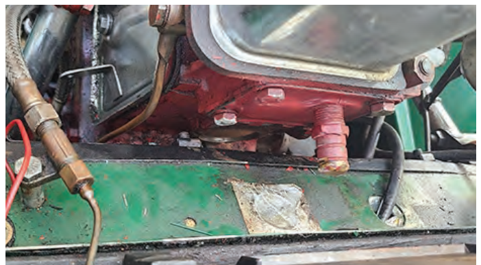
The replaced leaking freeze plug.
