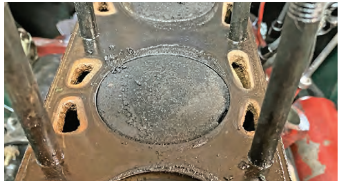
... we found a chip out of the suspect cylinder ...
