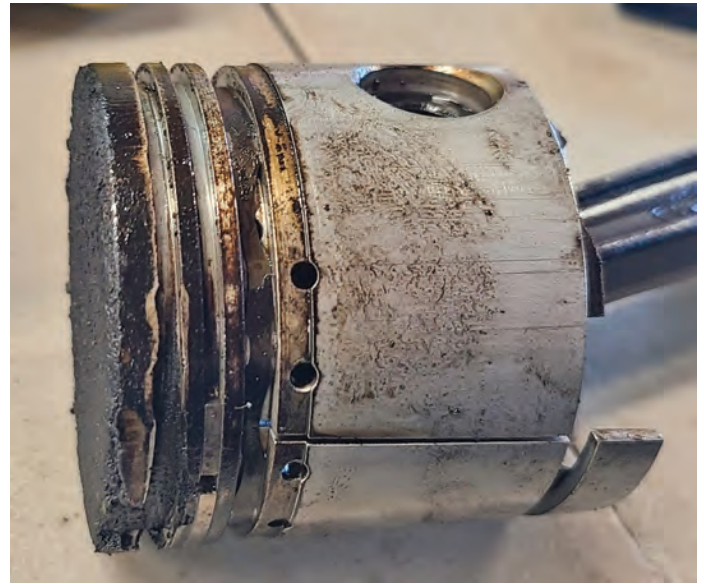
The damaged piston.
