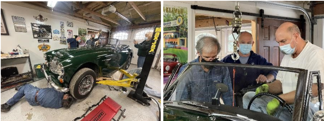
Dennis at the front controlling the floor jack supporting the transmission from underneath. A come-along attached to the roof rafters lifted the transmission from the top.
