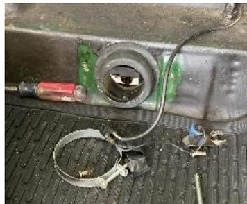
We unclamped the fuel pump from inside the trunk then pushed it through.
