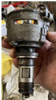
It was a struggle to get the distributor out of the engine. There was a lot of corrosion and moisture under the cap. The wire to the original electronic ignition were cut and an aftermarket installed. Now were putting a 3rd generation Pertronix ignition in.
