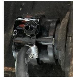
Determined it was a small crack near the hose connection.
