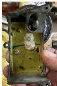
The base plate in the distributor was pretty corroded. The new Pertronix includes the base plate.
