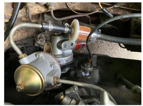
Removed and cleaned fuel lines from tank to fuel pump. Cleaned out 30 year old gasoline from tank and flushed out residue. Installed new fuel pump. Installed new oil filter adapter for a screw-on oil filter. Engine fires up and runs briefly. Need adjustments on dual 175 cfm Strombergs.
