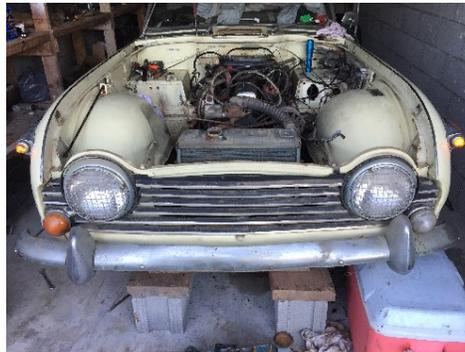
Bonnet off for radiator, water pump, thermostat, fan, and front oil pan seal inspection and repair. Closer to firing up 2.5L in-line six.
