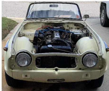
First time I drove the TR. Has new clutch, brakes, steering shaft yoke, ball joints, and tires. Drives well but needs suspension components. Will start with shocks and bushings being replaced, as I continue to drive and repair.
