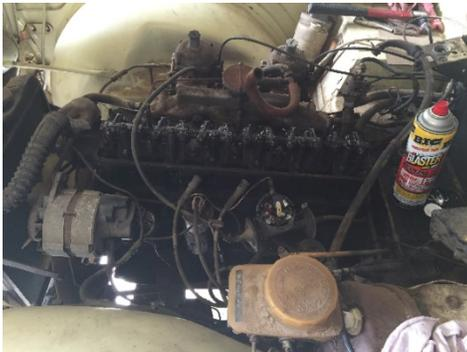
Turning engine over by hand after pulling spark plugs, checking valve lash, and using ATF and PB Blaster to lube cylinders.
