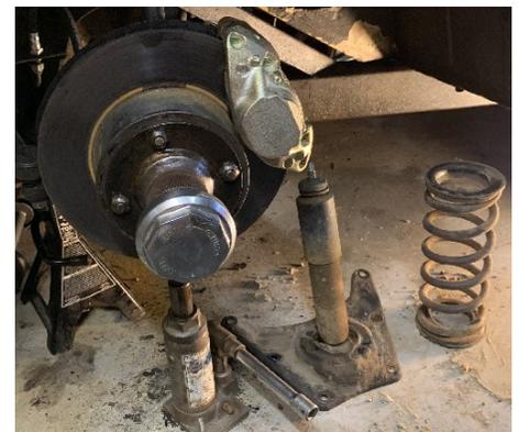
Front suspension - New shocks, coil springs, bushings to be replaced. The coil spring compressor was too large to fit in the space. The lower A frame was removed with the jacks and all just dropped out as jack was released. I ended up making a rod compressor. It worked well with long guide bolts in center holes on wishbone.
