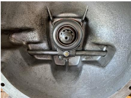
New clutch, pressure plate, Koyo release bearing, pilot bearing, clutch fork-new tapered pin (old one broken-common problem on TRs) drilled fork and rod and installed 1/4" bolt, a recommended modification.
