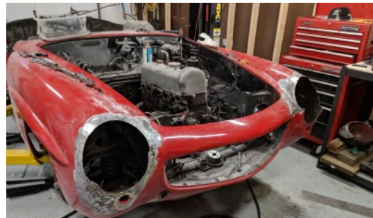
Old repairs were cut out. I have new buckets but need to make the fender metal.
