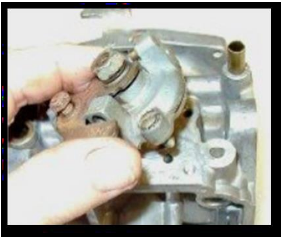
10. Remove the bypass valve assembly (three slotted screw) and the idle trim adjuster screw.
