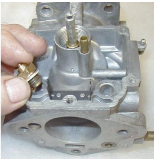
11. Remove the float bowl valve and aluminum washer.
