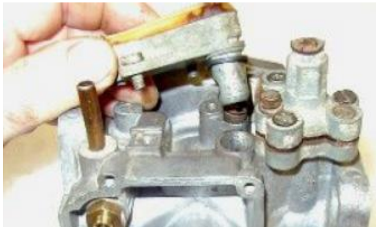
10. Remove the bypass valve assembly (three slotted screw) and the idle trim adjuster screw.
