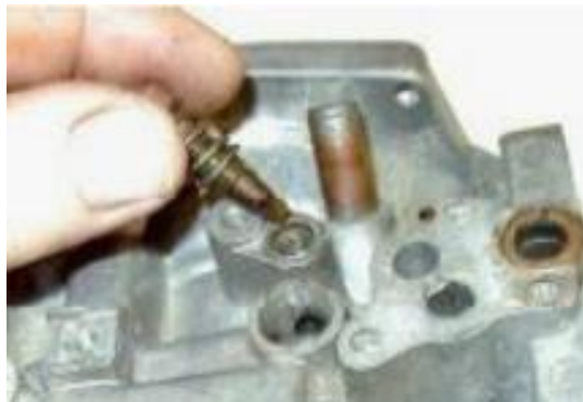
11. Remove the float bowl valve and aluminum washer.
