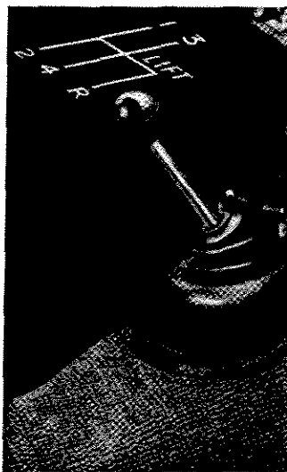
Fig. 10. Change speed lever positions
