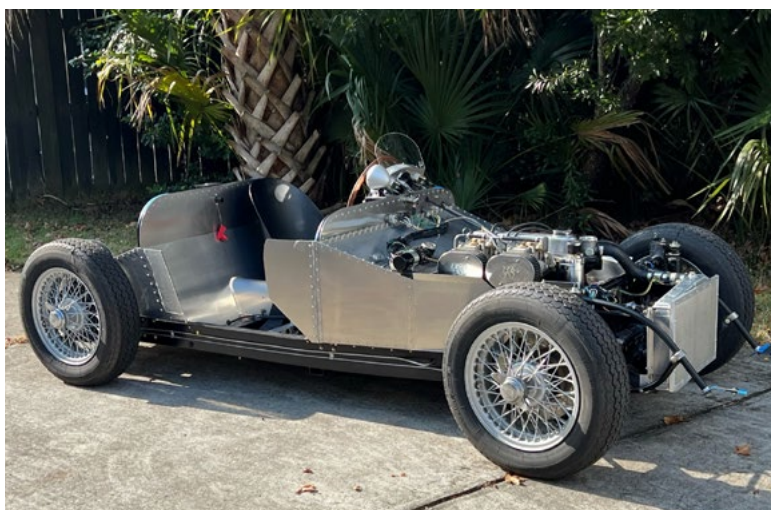
With the Devin body detached, the rolling chassis illustrates custom aluminum stiffening panel system with body location points. Note the builder's detailing, engineering, and meticulous fastener technique.
