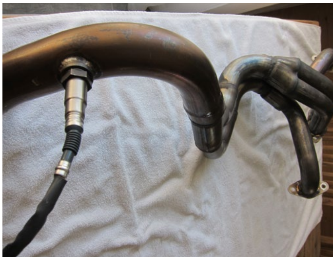
The oxygen sensor and its adapter installed in the exhaust manifold
