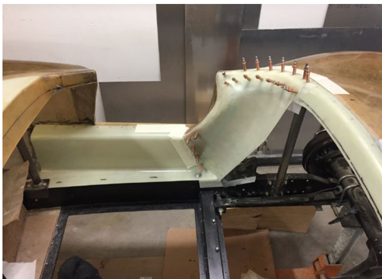
The fiberglass piece made from the aluminum mold being added to the body shell
