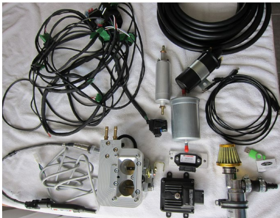
The contents of the Classic Fuel Injection kit
