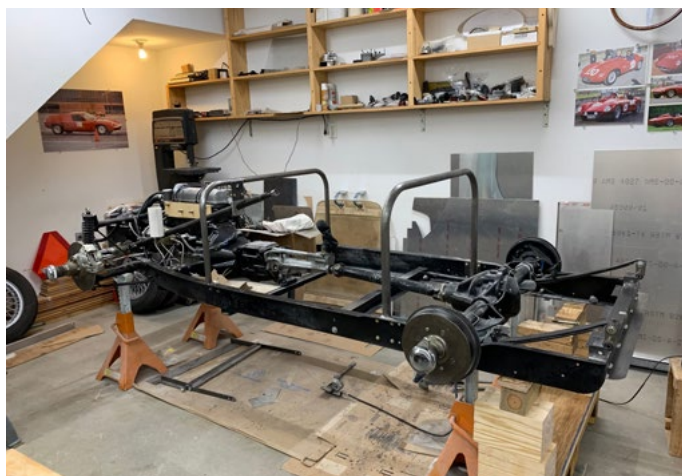
The Shortened chassis illustrates modified rear spring location and dimensions. Engine and driveline repositioned to align with differential
