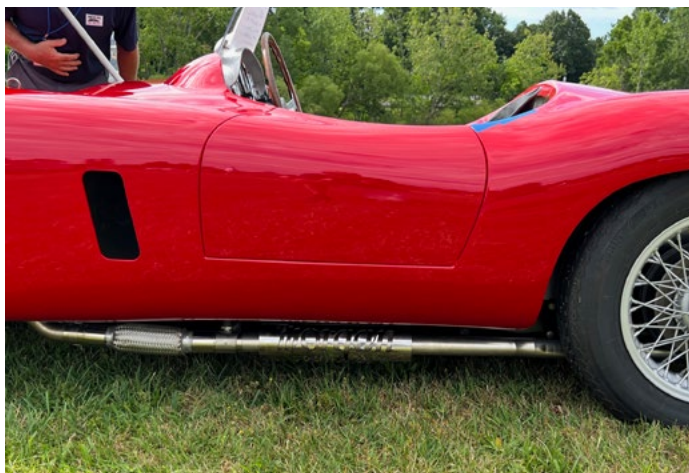
Ferrari-inspired exhaust with Morgan script heat shield
